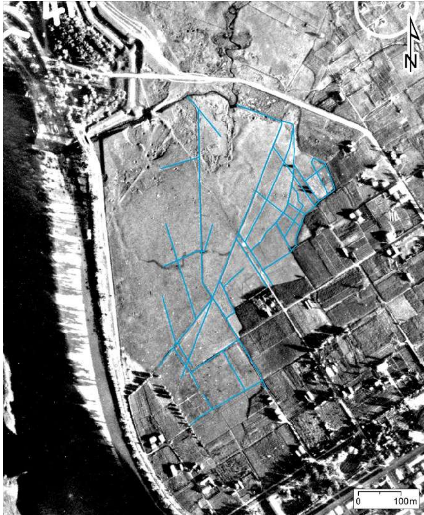
Figure 32 Luftwaffe (Nazi German Air Force) vertical aerial reconnaissance photograph taken in 1944 - with blue lines indicating the location of drainage ditches
